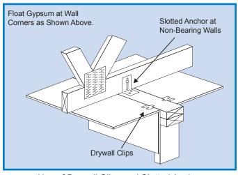
Use of Drywall Clips and Slotted Anchor on Non-Bearing Wall
