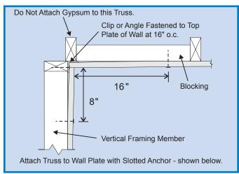
Floating Gypsum Corner II (Truss Parallel to Wall)
