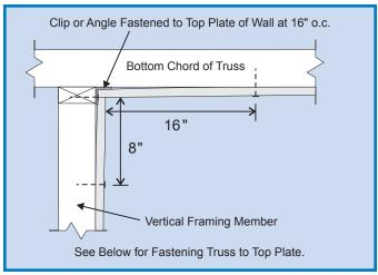
Floating Gypsum Corner I (Truss Perpendicular to Wall)
